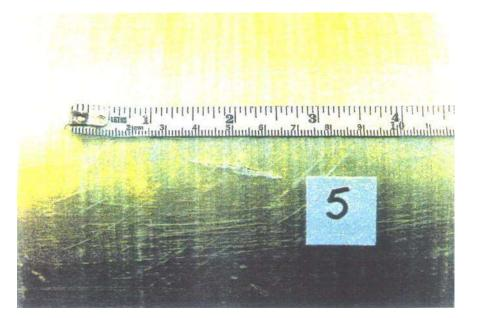
a) Level damage from cuts — Sperficial cut
