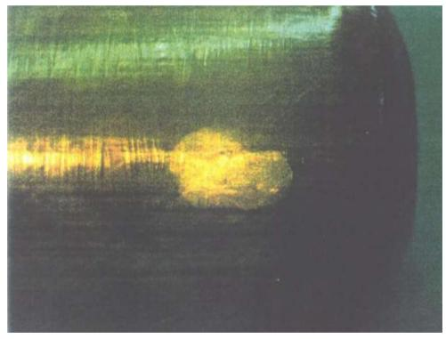
b) Level 3 impact damage — Depth of damage over 15 % of thickness (fully wrapped cylinder)
