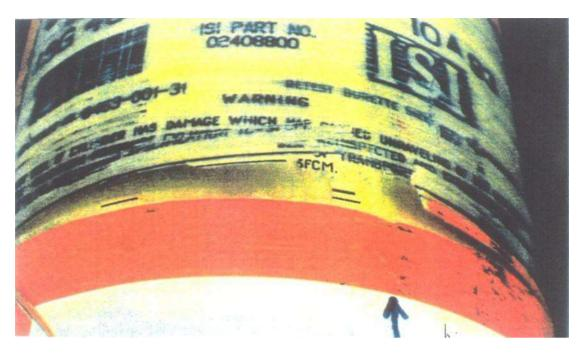
Figure 4 — Delamination
